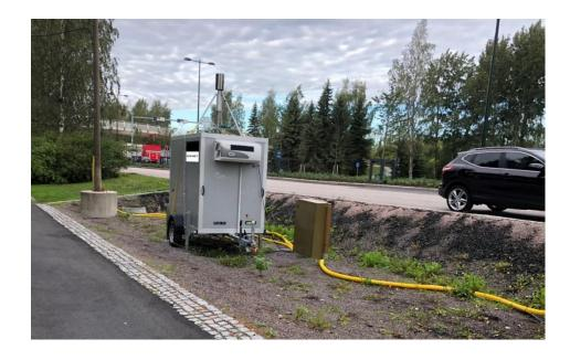
Sensmet monitoring station continuously analyses stormwater quality in a nonstop fashion, 24 hours a day.
